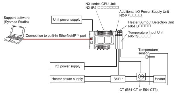
\* The SSR is used to turn the heater ON and OFF.
