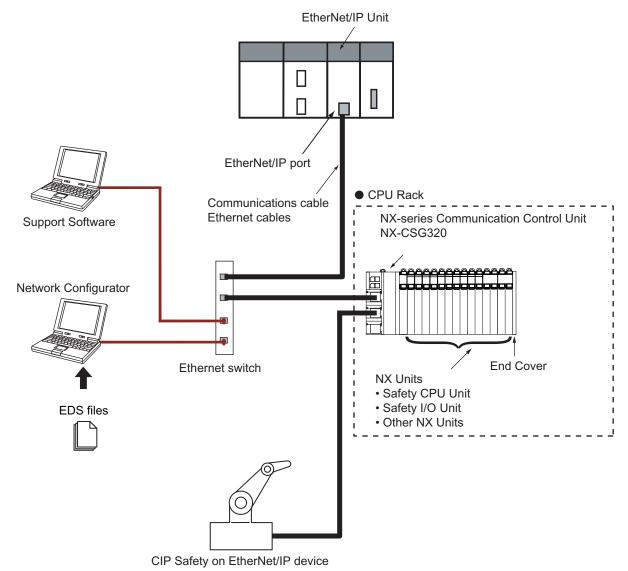
Note: For whether an NX Unit can be connected to the Communication Control Unit, refer to the version information.
