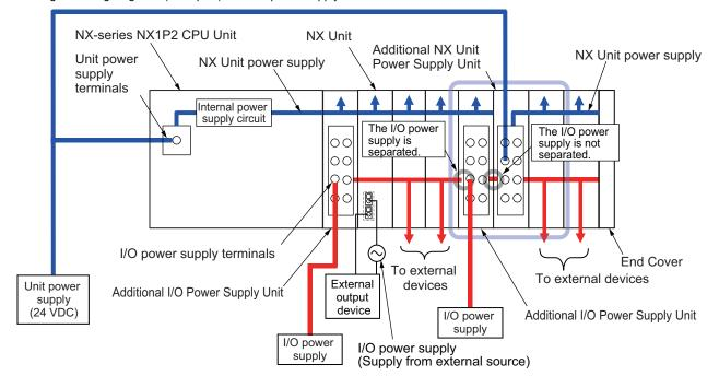
Note: Supply the Unit power and the I/O power from different power supplies. If you supply power from the same power supply the galvanic separation between the bus system and the I/O circuits is no longer effective. Noise generated in the I/O circuits may cause malfunctions in the internal circuits of the units.
