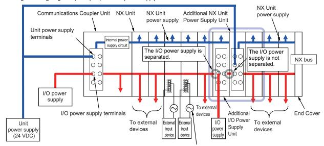
I/O power supply (Supply from external source)
