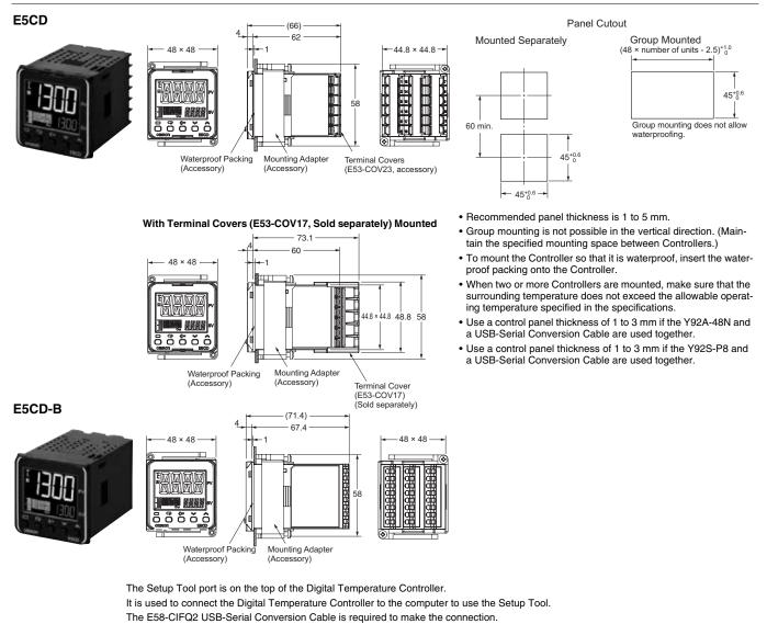
Refer to the instructions that are provided with the USB-Serial Conversion Cable for the connection procedure.
