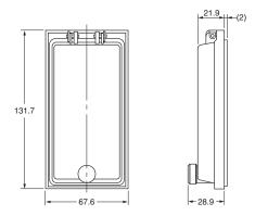
Draw-out Jig (Cannot be used on a Push-In Plus terminal block type) Y92F-59
