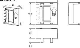
Terminal Covers (Cannot be used on a Push-In Plus terminal block type)
