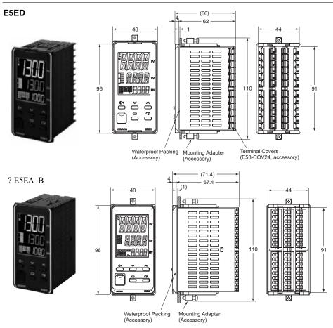
• Setup Tool ports are provided as standard feature. Use these ports to connect a computer to the Digital Temperature Controller. The E58-CIFQ2 USB-Serial Conversion Cable is required to connect to the port on the top panel. The E58-CIFQ2 USB-Serial Conversion Cable and E58-CIFQ2-E Communications Conversion Cable are required to connect to the port on the front panel. (You cannot leave either port connected constantly during operation.)
