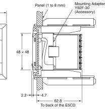
DIN Track Mounting Adapter (Cannot be used on a Push-In Plus terminal block type) Note: This Adapter cannot be used together with the Terminal Cover. Y92F-52 Remove the Terminal Cover to use the Adapter.
