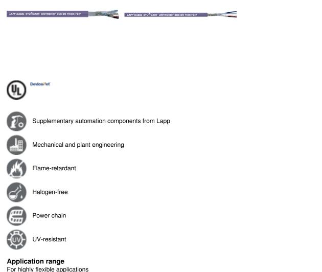
For highly flexible applications DeviceNet<sup>™</sup> connects industrial devices e.g. limit switches, photoelectric switches, valve islands, motor starters, drives, PLCs, etc.
