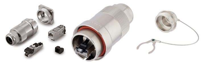
**Product features** Housing: brass nickel plated Qualified for 10 Gigabit/s Ethernet Suitable for stranded cores with AWG27/7 -22/7 and for solid conductors with AWG26/1- 22/1
