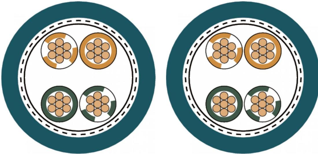
LAPP KABEL STUIGART ETHERLINE® Y Flex CAT.5e 4x2xAWG26/7
