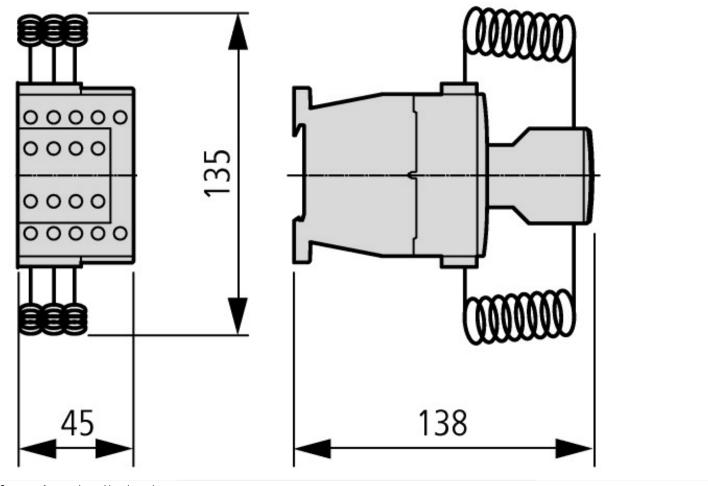
Contactors for capacitors with series resistors
