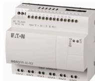
**Control relay, 100-240VAC, 12DI, 6DO relays, time, expandable, easyNet**
