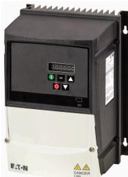
**Variable frequency drive, 400 V AC, 3-phase, 4.1 A, 1.5 kW, IP66/NEMA 4X, Radio interference suppression filter, Brake chopper, 7-digital display assembly, Local controls, Additional PCB protection, UV resistant, FS2**
