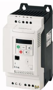
**Variable frequency drive, 230 V AC, 1-phase, 10.5 A, 1.1 kW, IP20/NEMA 0, Radio interference suppression filter, Brake chopper, FS2**
