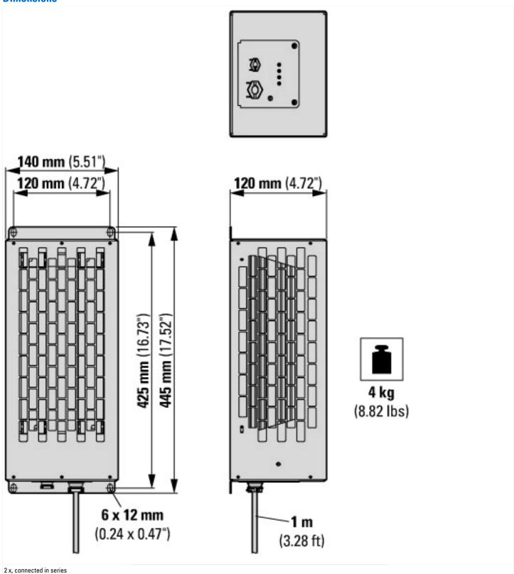
2 x, connected in series Mounted as required
