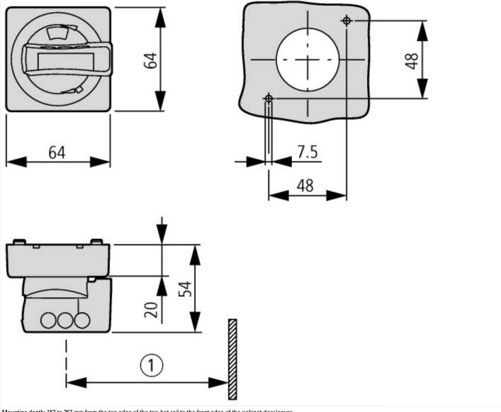
Mounting depth: 152 to 267 mm from the top edge of the top-hat rail to the front edge of the cabinet door/cover ① At least 100 mm from cover hinge
