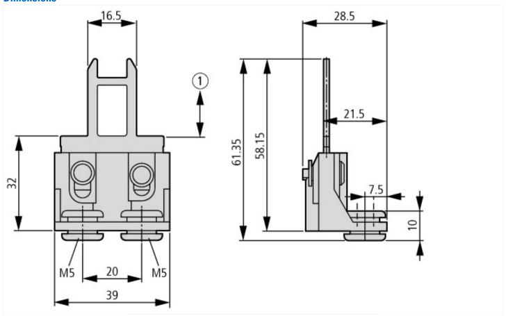
Fixing only allowed with M5 fixing screw and washer according to DIN EN ISO 7093 1 Distance to device head = 0.1  $\dots$  3.0 mm
