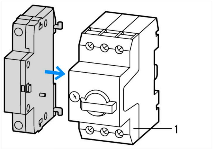
1: Motor-protective circuit-breakers
