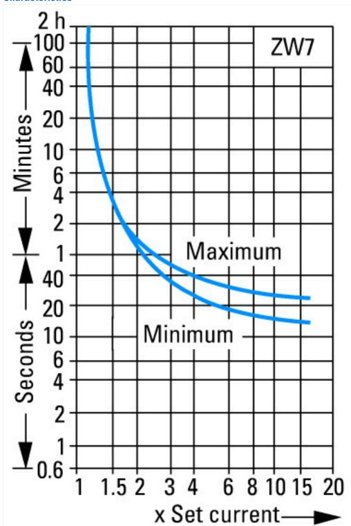
These tripping characteristics are mean values of the spread at 20 °C ambient air temperature in a cold state. Tripping time depends on response current. When the devices are at operational temperature the tripping time of the overload relay reduces to approx. 25 % of the read off value.
