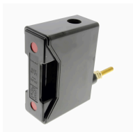
Fuse-holder, low voltage, 100 A, AC 690 V, BS88/A4, 1P, BS
