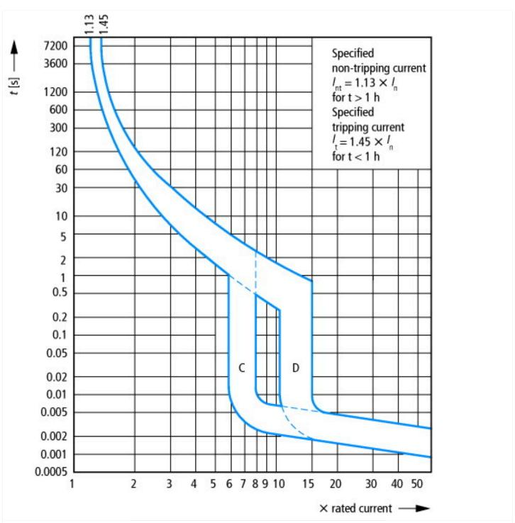
Tripping characteristic at 30 °C: C, D according to IEC/EN 60898
