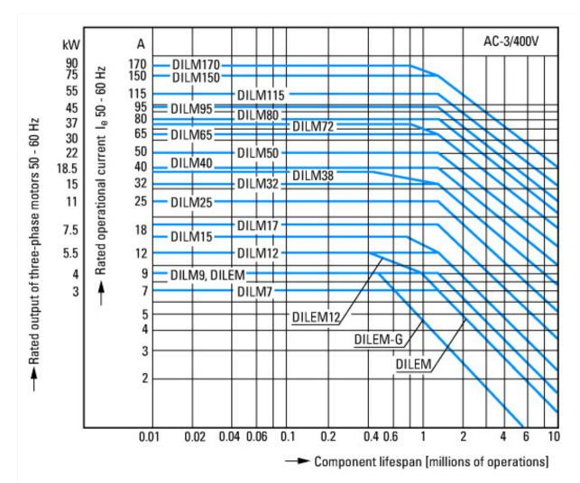
Squirrel-cage motor Operating characteristics Starting:from rest Stopping:after attaining full running speed Electrical characteristics Make: up to 6 x rated motor current Break: up to 1 x rated motor current Utilization category 100 % AC-3
