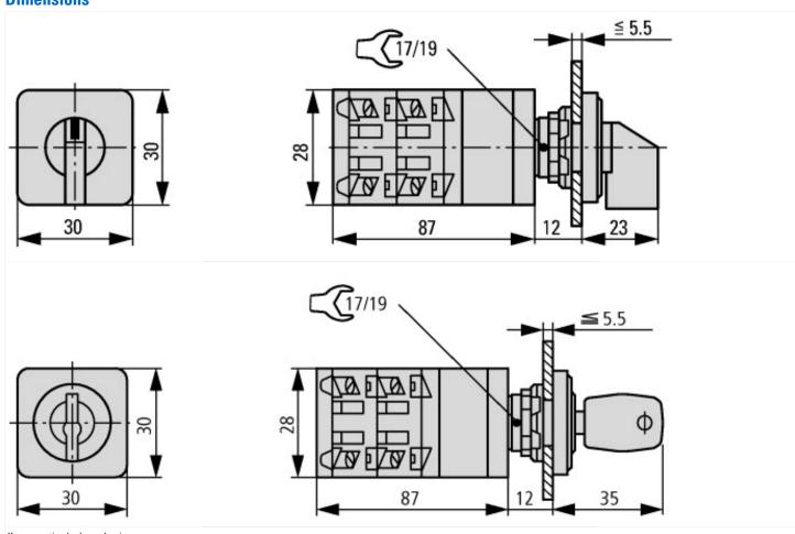
Key operation lock mechanism
