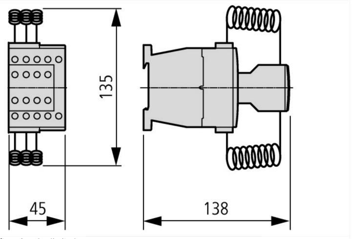
Contactors for capacitors with series resistors
