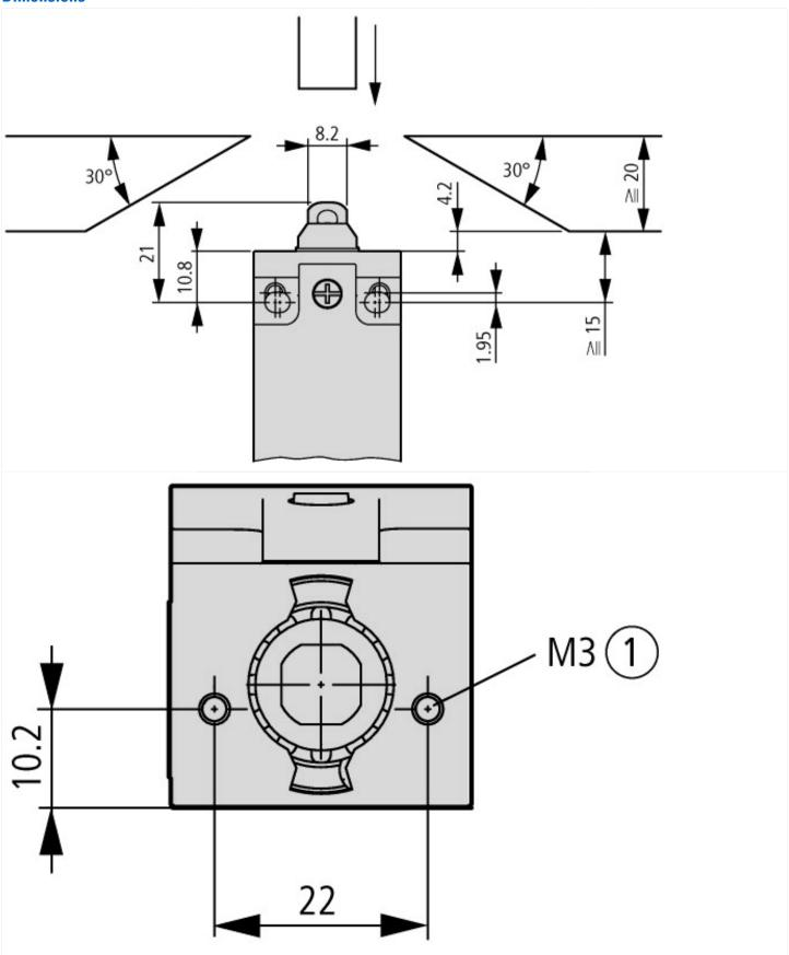
① screw-in depth max. 12 mm
