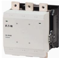
**Contactor, 380 V 400 V 560 kW, 2 N/O, 2 NC, RAC 500: 250 - 500 V 40 - 60 Hz/250 - 700 V DC, AC and DC operation, Screw connection**
