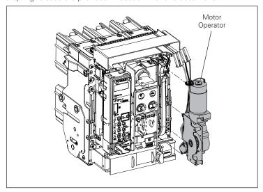
Figure 15. Motor Operator Location.
