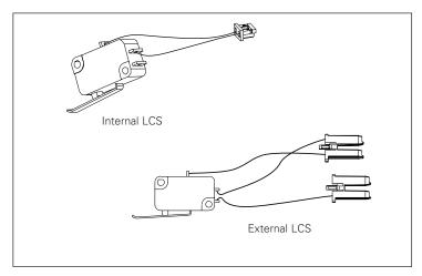
Figure 2. Latch Check Switches.
