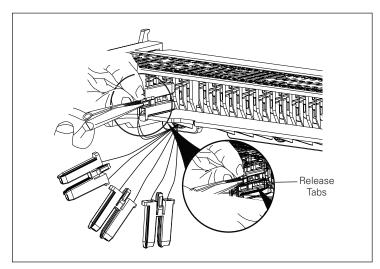
Figure 31. Connector Plug Removal.
