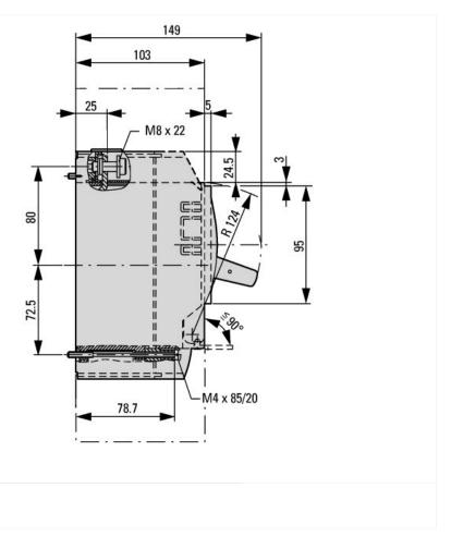
Blow out area, minimum clearance to other parts ≥ 90 mm
