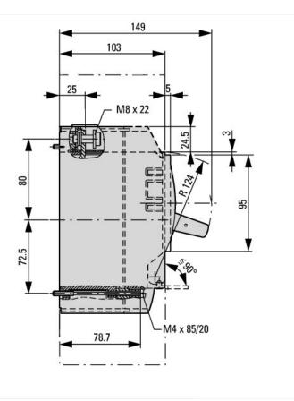
Blow out area, minimum clearance to other parts ≥ 90 mm
