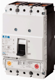
Circuit-breaker, NZM1 TMTU, 3 pole, 32A, box terminal
