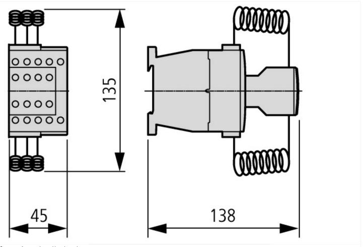
Contactors for capacitors with series resistors
