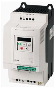
Variable frequency drive, 230 V AC, 3-phase, 24 A, 5.5 kW, IP20/NEMA 0, Radio interference suppression filter, 7-digital display assembly
