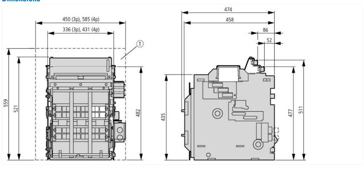
① Recommended minimum enclosure size (not shown to scale)
