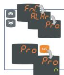
After pressing the "fnc" key, the UP and DOWN keys can be used to scroll through the folders in the menu
