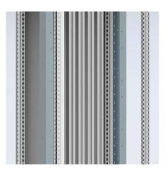
**Descrição:** Vertical busbar to build up the plug-in system. The MSBS bars are fixed in the MSVH supports with standard bolts, washers and nuts. The rated current can be increased up to  $2 \times 1400A$  if the incoming connetion is in the middle.
