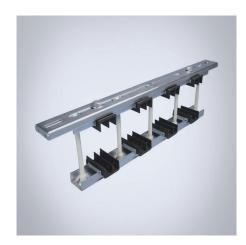
**Descrição:** Busbar support up to 4500A to be mounted horizontally or vertically. Mounts directly to the enclosure frame or with help of CLPF profiles. Available in one/ two/three bars per phase for bar thickness 10 mm, and width from 30 to 120 mm.
