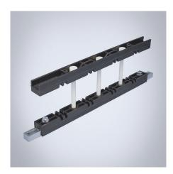
**Descrição:** Busbar support up to 1600A to be mounted horizontally or vertically. Mounts directly to the enclosure frame or with help of CLPF profiles. Available in single and double bar per phase for bar thickness 5 mm and only single bar per phase for bar thickness 10 mm, and width from 25 to 80 mm.
