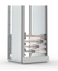
**Description:** Support to be mounted horizontally in the enclosure. Is mounted to the internal side panels, MSPS, and the enclosure frame. Makes it possible to mount the MSHS busbar support in depth in a horizontal position. Ideal when there are many incoming/outgoing cables and need a horizontal connection.
