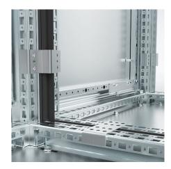
**Description:** Baying brackets provide a rigid reinforcement of the enclosure assembly. The correct spacing between the enclosures is assured. Tools are not required for installation.
