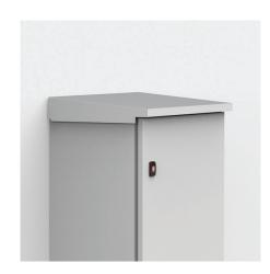
**Descripción:** To be fitted as an outdoor shelter on single mounted enclosures. The roof is slightly sloped and has a dripstrip. Machining is required. It increases the enclosure dimension in H:60 mm, D:20 mm and W:20 mm.
