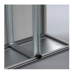
**Description:** Fitted in the centre of a 1200 mm or 1600 mm wide enclosure (top and bottom), to provide standard mounting facilities in two sections of 600 mm or 800 mm wide. This enables separate fitting of accessories such as CAB(P), CBU, CLPK, CLPF etc., in either side of the enclosure. Accessories are adjustable in depth within the 25 mm hole pattern.
