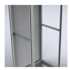
**Description:** Profiles for partial and full depth mounting of the telescopic shelf SHT. Makes possible to mount a 600 mm deep SHT in a 800 mm deep enclosure. Fixed directly to the enclosure's frame. Fully adjustable in height in steps of 12.5 mm.
