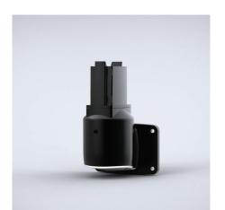
**Description:** Wall joint with vertical outlet component for SM system, angle of rotation 300° with stop. Rotation angle limiter is to be ordered as a separate product. Cable access with a plastic screw fitted cover.
