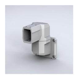
**Description:** Wall joint with horizontal outlet component for SL system, angle of rotation 300° with stop. Rotation angle limiter is to be ordered as a separate product. Cable access with a plastic click-in cover.
