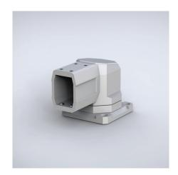
**Description:** Set-up joint component for SL system, angle of rotation 300° with stop. Rotation angle limiter is to be ordered as a separate product. Cable access with a plastic click-in cover.
