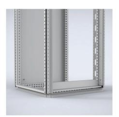
**Description:** Two single vertical profiles, which can be used both for front covers and assembly of components. A cost effective solution for panel builders, reducing assembly time, which also enables assembly outside the enclosure. Useful height for front covers is, Height – 150 mm.
