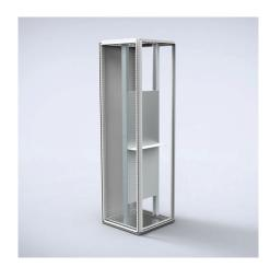
**Description:** Pre-sized horizontal separation plates between the mounting level and the front covers. Slides easily into place and let us to get Form 4 compartments for MCB's and MCCB's. No screws need.
