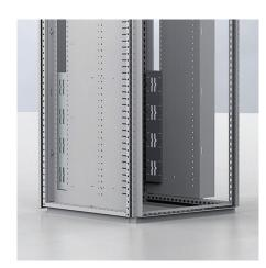
**Description:** Busbar supports up to 3600A to be mounted horizontally behind the compartments. Mounts to the internal side panels MSPS, and in the height position which we need. Supports for single or double bar per phase for bar thickness 10 mm, and width from 10 to 120 mm. Distance between bars of 20 mm.
