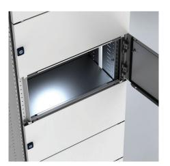
**Description:** Pre-sized horizontal separation plates between the mounting level and the front door. Slides easily into place and let us to get Form 4 compartments for MCB's and MCCB's. No screws need.
