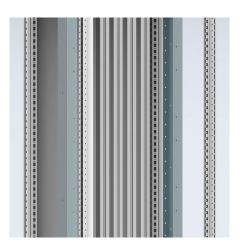
**Description:** Vertical busbar to build up the plug-in system. The MSBS bars are fixed in the MSVH supports with standard bolts, washers and nuts. The rated current can be increased up to  $2 \times 1400A$  if the incoming connetion is in the middle.
