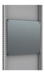
**Description:** Mounted directly on the enclosure's frame or onto the clickin profiles (CLPK). Special design of the bracket allows one man assembly. Can be mounted in any height or depth position within the 25 mm hole pattern. Appropriate sizes can also be used on the sides of the enclosure.
