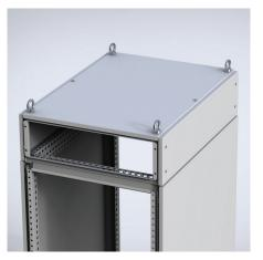
**Description:** For cable entry and routing or for installation of a power distribution system. Fixed to the top of the enclosure by four M12 screws. Available in 200 mm and 300 mm heights. The enclosure roof plate CCR can be used to close the top. For lifting a 200 mm high MCU together with an enclosure a separate lifting kit MCUK is needed. 300 mm high MCU's must be lifted separately.
