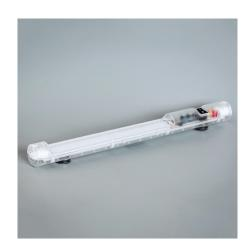
**Description:** Energy saving lighting system suitable for all types of panels and enclosures, especially where space is at a premium. It is made of transparent plastic. This lamp has a very long service life (around 60,000 h.) thanks to the use of LED technology. The power output allows up to 10 lights to be connected to each other (daisy chain) with both the input and output plugs snap-locking into their sockets.
