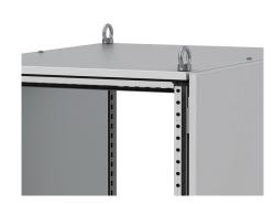
**Description:** Mounts directly to the frame corner pieces of the enclosure for when lifting operations are required. Complies with DIN 580 lifting requirements. M12 thread.
